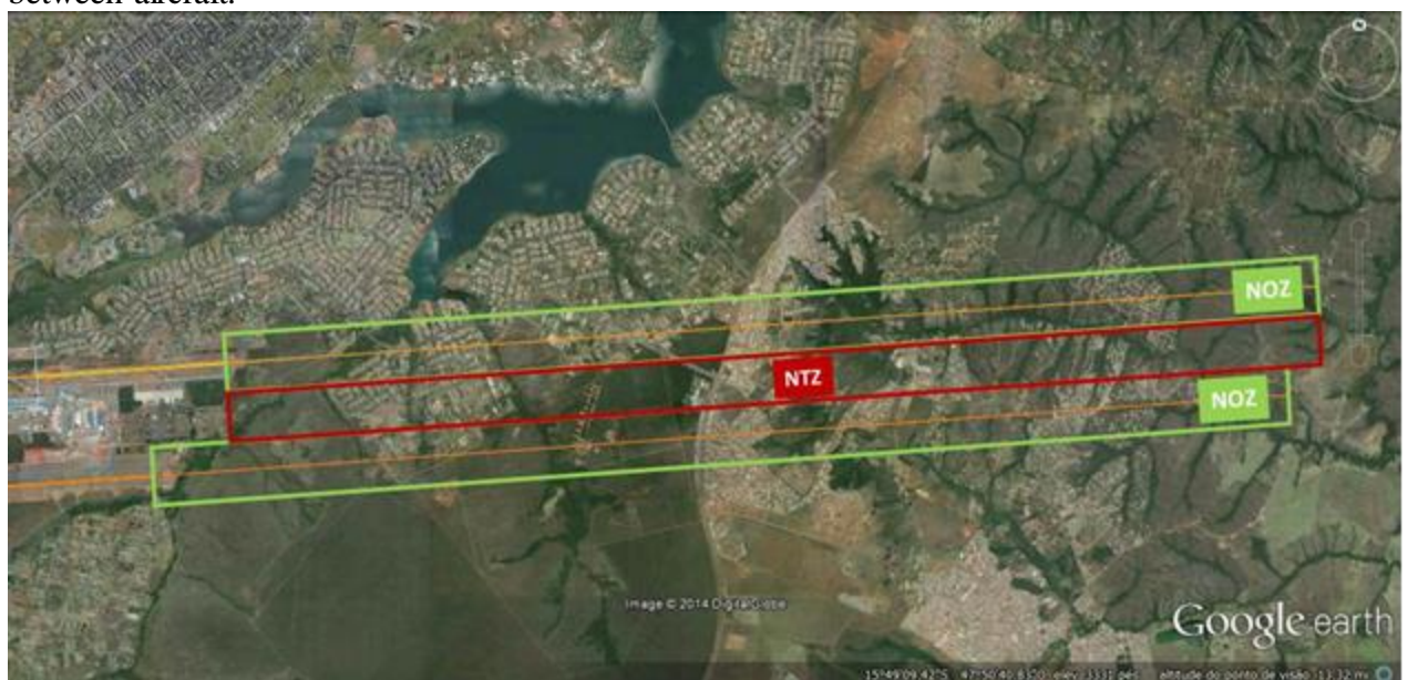
Figure 1: SBBR RWY 29 NTZ and NOZ Configuration
