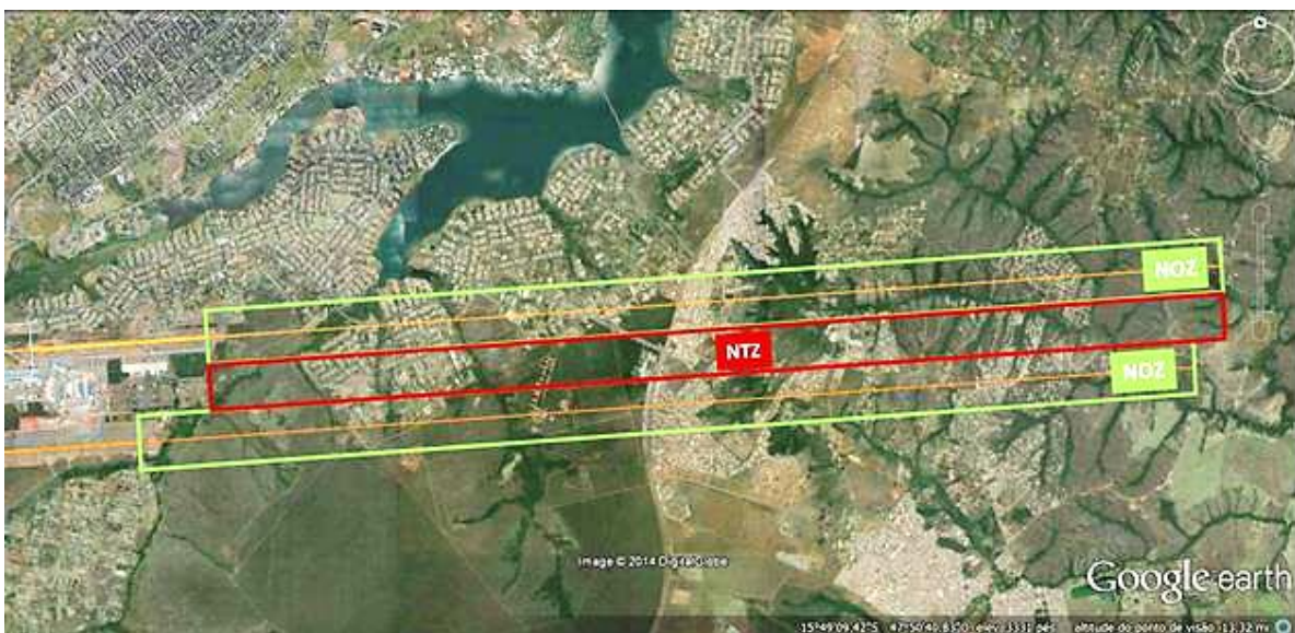
Figure 1: NTZ and NOZ configuration of SBBR runways 29
